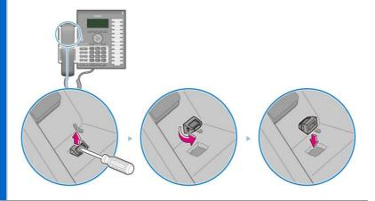
Attach to match wall mount bracket hole and screws, and pull down to make sure firmly fixed.
