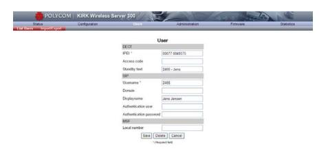
The data configured for each handset can be split into two categories. DECT data which is necessary for the correct handling of the DECT protocol stack. SIP data which is necessary for the handling of a SIP user agent.
