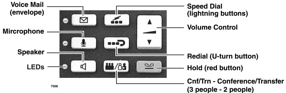
**Note** The IPT Fixed Buttons work the same way as the DKT telephones, however on the IPTs, fixed buttons have been replaced with button icons.
