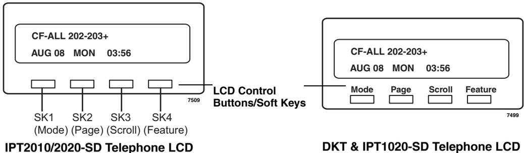
**Note** The IPT and DKT soft keys perform the same functions. This manual uses the IPT soft keys (SK) to refer to the soft keys on all telephones. For example, if an instruction references SK1, this means use the first soft key (from left to right) on the IPT and use Mode on the DKT. SK2, SK3 and SK4 equate to the second, third and fourth soft keys on the IPT or Page, Scroll and Feature on the DKT.
